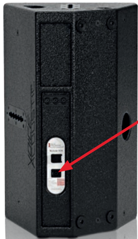
Modular-15 bi-amping 15" on CH1, 2.400 W, Speakon 2+/2- 1,4" on CH2, 800 W, Speakon 1+/1-
