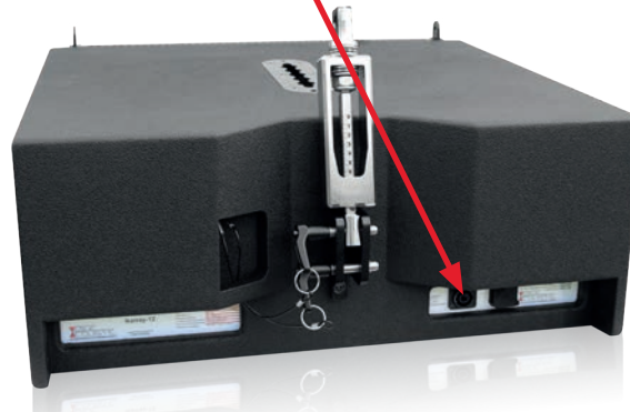
Ikarray-12 bi-amping 12" on CH1, 2.400 W, Speakon 2+/2- 1,4" on CH2, 800 W, Speakon 1+/1-
