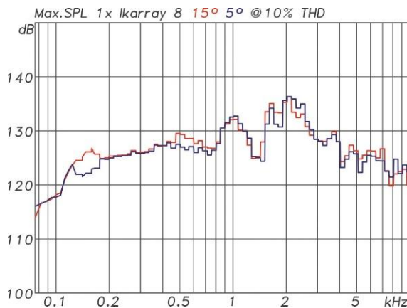
Maximum spl for maximum 10% distortion for a single Ikarray-8 system with 15° angle (red) and 5° angle (blue). The measurement was performed with 185 ms long sinus bursts (Fig. 16)
