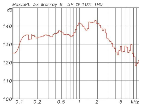
Maximum spl for maximum 10% distortion for an array of three systems with 5° beam angle. The measurement was performed with 185 ms long sinus bursts (Fig. 17)
